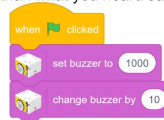
Adjust the pitch of the buzzer by using the code "change buzzer by ()".
