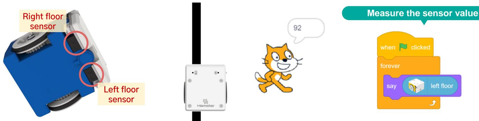
The Say code can be used to measure the floor sensor values.
